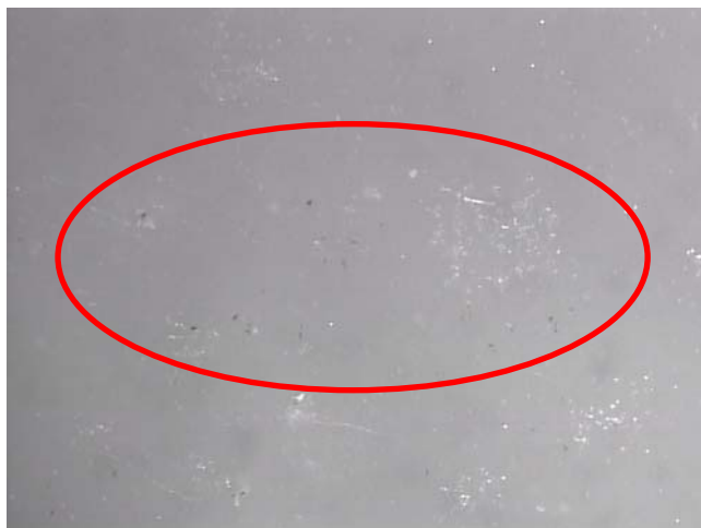
Photo 2: Material Würth Acetatsilikon Lebensmittel , color transparent/ whity after an incubation period of 28 days with low fungal growth (at a magnification of x 50)
