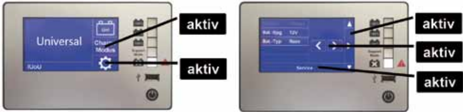
Fig. 6: Control panel: Active areas
